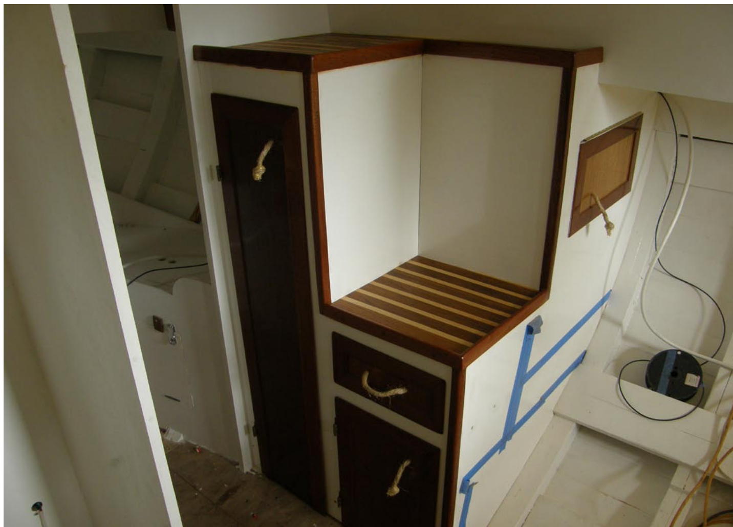
The storage lockers in the main cabin have new molding all around and a fresh coat of varnish.
