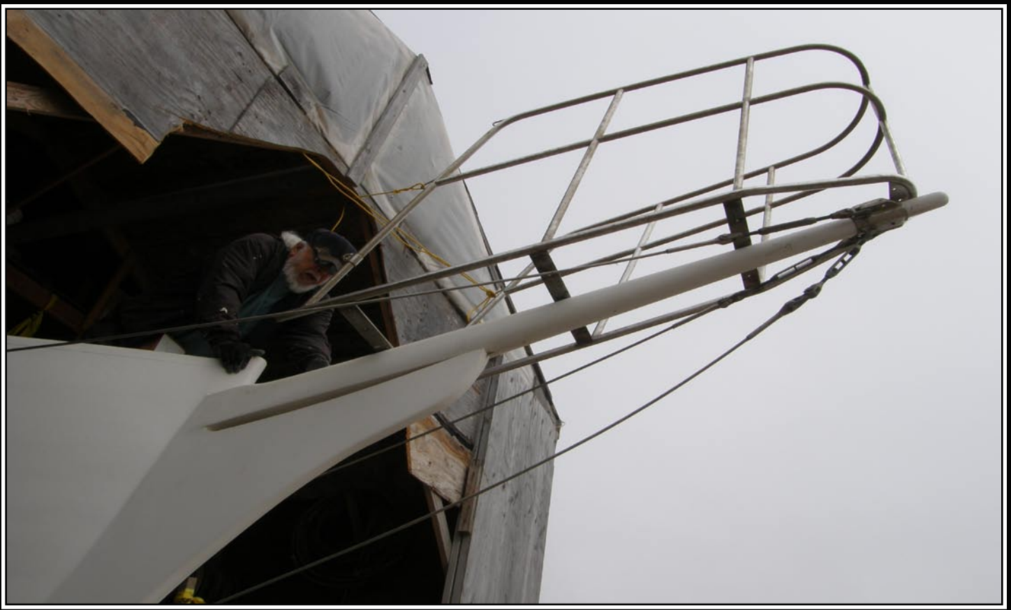
Mike is now working on the pulpit, that's the small cat walk looking thing that juts out over the bow sprit on the forward most part of the boat.
